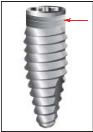
Fig 1 The Laser-Lok collar of a dental implant. The red arrow distinguishes the upper zone, which consists of 8- \mu m microchannels that are 6 \mu m deep, from the lower zone, which consists of 12- \mu m microchannels that are 12 \mu m deep.
